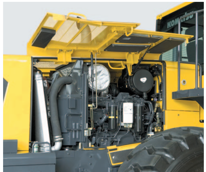
Gull-wing side doors upper stop position
