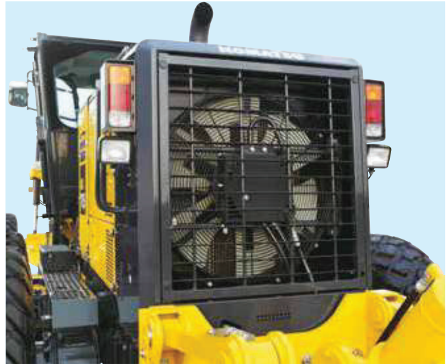
Hydraulic driven cooling fan
