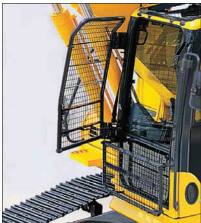
Cab front full height guard level 1 (ISO 10262)
