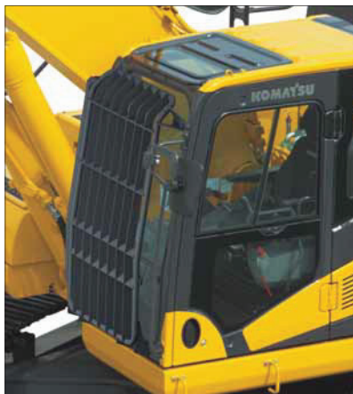
Cab front full height guard level 2 (ISO 10262)
