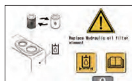
Clogging hydraulic oil filter caution
